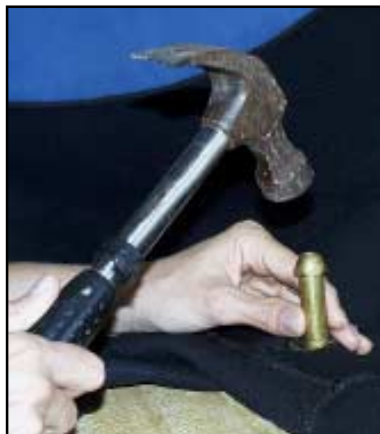
USING A PUNCH TO MAKE A HOLE -PREFERRED METHOD-
