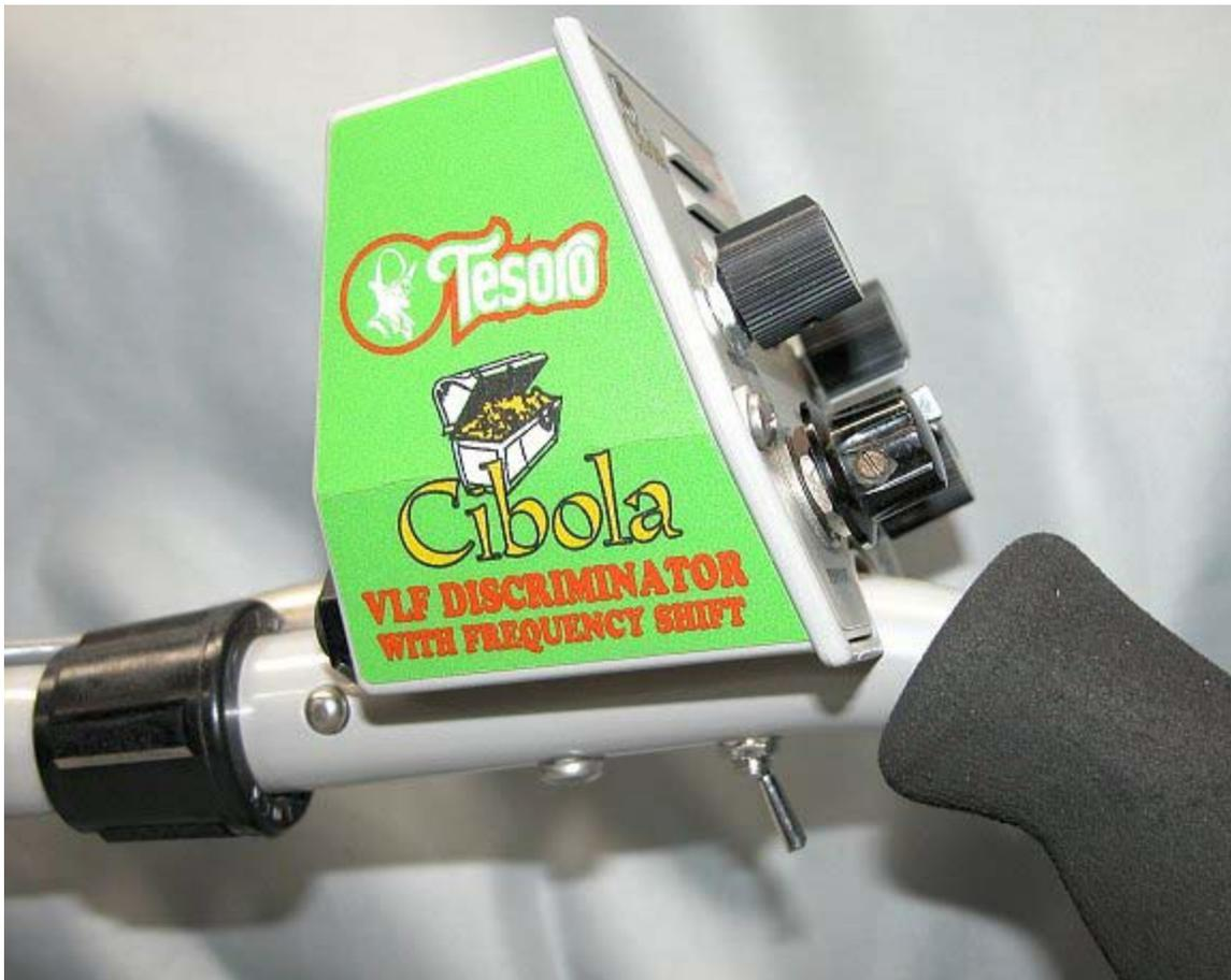
Time to replace your control knobs. I put some small o-rings underneath them to keep dirt, etc out of the pots. As well as to put slight tension on the GB and Threshold controls. Less chance for them to be accidentally bumped changing your GB setting.
