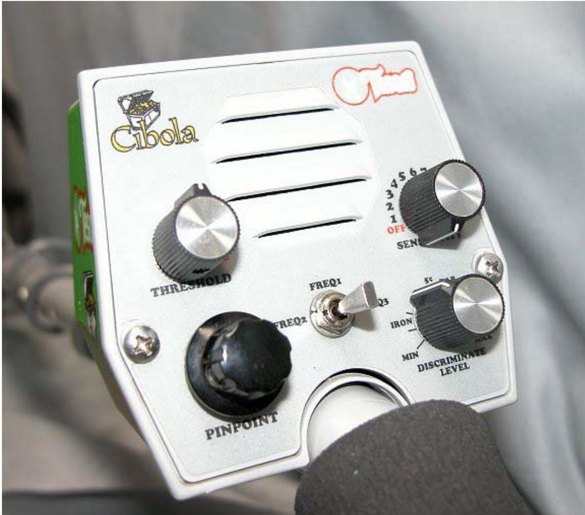
You can use any knobs you like, matching or otherwise. The bourns pot has a  $\frac{1}{4}$ " round shaft, so any knob that is made for  $\frac{1}{4}$ " shafts can be used. I had one laying around from an old Garrett detector and used it for the GB. When I get around to it my Cibola will have all matching knobs.
